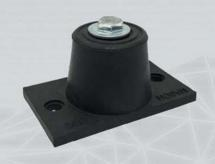
**Type ND** with rubber is loaded in both shear and compression to provide rubber in shear performance as well as overload protection. They are one piece molded assemblies with skid resistant rubber ridged base plates and circular rubber ridged tops. The complete neoprene covering of the metal parts provides corrosion protection in either humid indoor or outdoor service.
